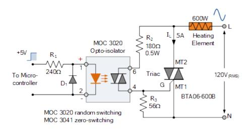
This type of optocoupler configuration forms the basis of a very simple solid state relay application which can be used to control any AC mains powered load such as lamps and motors. Here we have used the MOC 3020 which is a random switching isolator.
