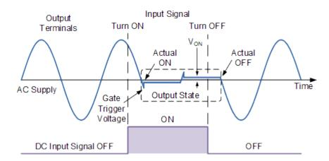
With no input signal applied, no load current flows through the SSR as it is effectively OFF (open-circuited) and the output terminals see the full AC supply voltage. With the application of a DC input signal, no matter which part of the sinusoidal waveform, either positive or negative the cycle is going through, due to zero-voltage switching characteristics of the SSR, the output only turns-on when the waveform crosses over the zero point.
