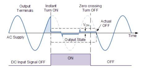
While this allows for the phase control of the load waveform, the main problem random turn-on SSR's is that the initial load surge current at the instant the relay turns-on, may be high due to the SSR switching power when the supply voltage is close to its peak value (900). When the input signal is removed, it stops conducting when the load current falls below the thyristors or triacs holding current as shown. Obviously for a DC SSR, the ON-OFF switching action is instant.
