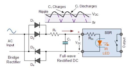
Bridge rectifiers convert a sinusoidal voltage into full-wave rectified pulses at twice the input frequency. The problem here is that these voltage pulses start and end from zero volts which means that they will fall below the minimum turn-on voltage requirements of the SSR's input threshold causing the output to turn "on" and "off" every half cycle.
