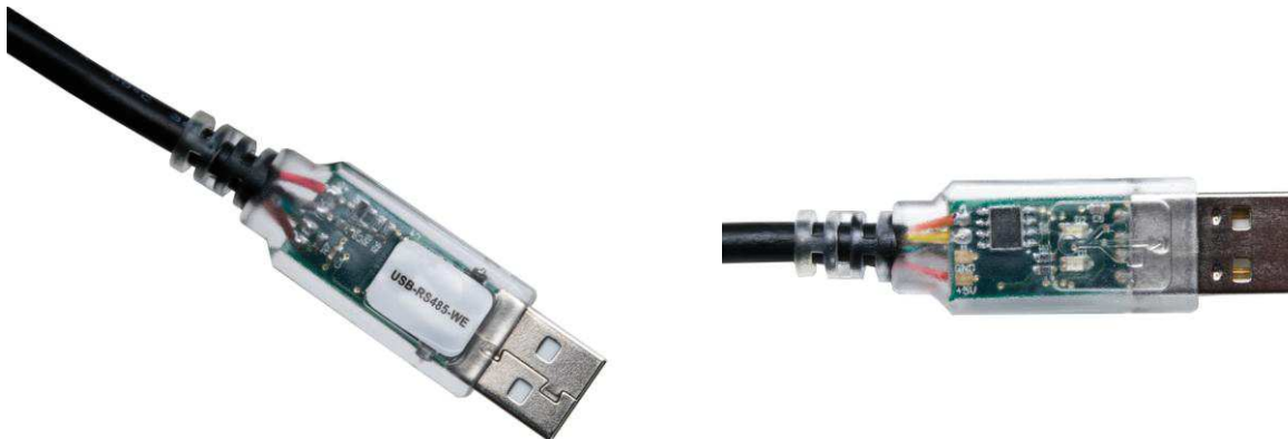
Figure 5.3 USB-RS485 Cable images
