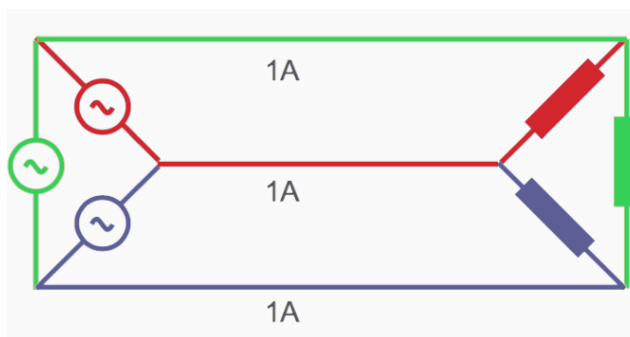
Figure 7 – Delta connection – three phase, three wires
