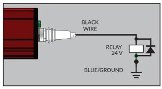
External relay can be connected for additional control/feedback configurations.
