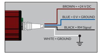
If remote monitor function is not needed insulate black wire and do not connect anything to it.
