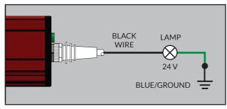
External indicator can be connected to BLACK wire to show status. This is useful for bars mounted in inaccessible areas.
