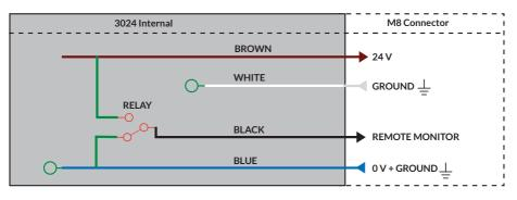
Remote Monitor signal is valid 4 seconds after power is applied.
