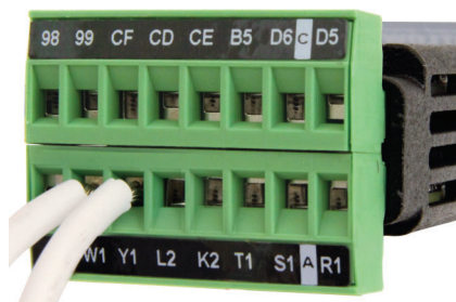
Figure 5: Switched DC Output Wiring
