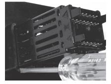
Place the blade of a screwdriver in any of the corner of the mounting collar assembly.
