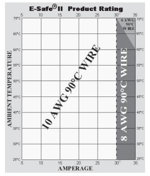
These ratings apply to 3-phase units with cycle times of 30 seconds or more. Consult the factory for 1- and 2-phase unit ratings.
