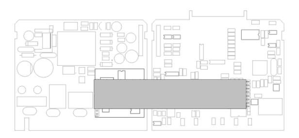
Once the Modbus module is installed, the communications are accessible from terminals 11,12 and 13 (see section 2.2).
