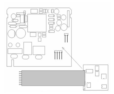
Plug the other Modbus module connector to the  $\mu400\text{P}/\mu500\text{PT}$  CPU board as shown in the figure below.
