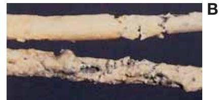
In an accelerated scaling test, researchers operated a 6000 watt FIREBAR heater side-by-side a 6000 watt, 0.315 in. (8 mm) round tubular element in a water heating application. Researchers added dehydrated lime to the water each day to accelerate scaling. Within four days, the scale on the round tubular element (heater B above) was thick enough to cause failure. The scale had built up to a thickness of 1/16 in. (4.1 mm), completely encompassing the sheath. The FIREBAR heater (heater A above) showed no signs of significant scaling other than small patches less than 1/32 in. (8.1 mm) thick. The majority of scale was flaking off the heater.
