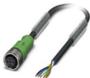
Sensor/actuator cable, 5-position, PVC, black RAL 9005, free cable end, on Socket straight M12, coding: A, cable length: 10 m
