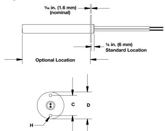
Stainless steel flanges are a convenient mounting method and can be used to position a heater within an application. The standard location is <sup>1</sup>/<sub>4</sub> in. (6 mm) from the lead end. However, a specific location may be requested in any location along the no-heat section. Unless specified, flanges are staked to the sheath.
