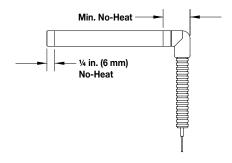
The diameter of the right angle extension is equal to the nominal diameter of the heater.
