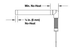
The diameter of the right angle extension is equal to the nominal diameter of the heater.
