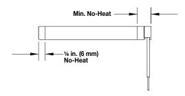
Right angle leads are used in applications with a high degree of flexing and when space limitations are critical. Standard lead wires are connected internally (swaged-in) and exit at a 90° angle at the end of the heater.
