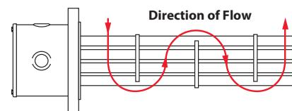
For forced circulation applications, 316 stainless steel baffles can be arranged on the heating element bundle to enhance and/or modify fluid or gas flow for better heat transfer.
