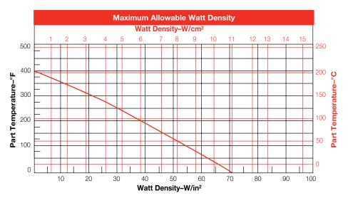
**Note:** The maximum watt density (W/in<sup>2</sup>) in open air is 5 W/in<sup>2</sup>. The chart above assumes bonding the polyimide heater to a part.
