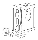
Many three-dimensional shapes, such as cylinders, cones and boxes, can be factory formed. Semi-rigid shapes can self-grip to the part. Special tooling may be required for some designs.
