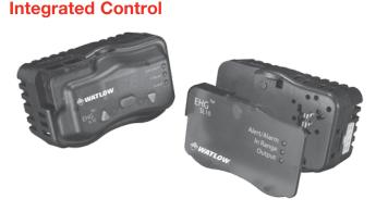
The SERIES EHG® is an integrated multi-function controller that is a key component in a powerful system that integrates a heater, an adjustable set point temperature controller, a high/low temperature alert, a power switching device and a high temperature safety limit. The agency recognized controller/safety limit meets UL® and CE requirements.
