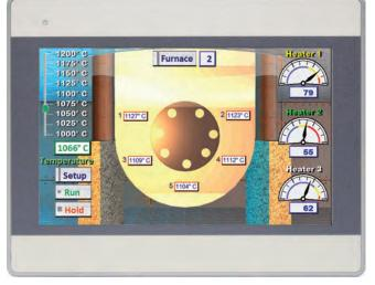
Include the types of displays users understand such as gauges, sliders and bar graphs to make screens intuitive.
