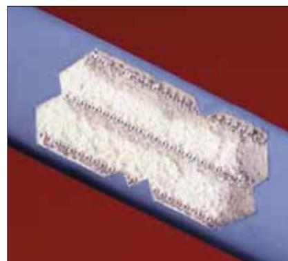
*For 240VAC, 10kW wiring, only the outside coils of a FIREBAR would be wired, each coil providing 5kW. For 208VAC, 10kW wiring, all three coils would be wired; the outside coils providing 3.75kW each and the different resistance center coil 2.5kW.*
